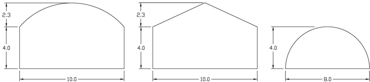
Fig. 2. Structural designs implemented in the greenhouse environment simulator. All three designs have 30 m of length, and are singlespan. Units are in meters.
