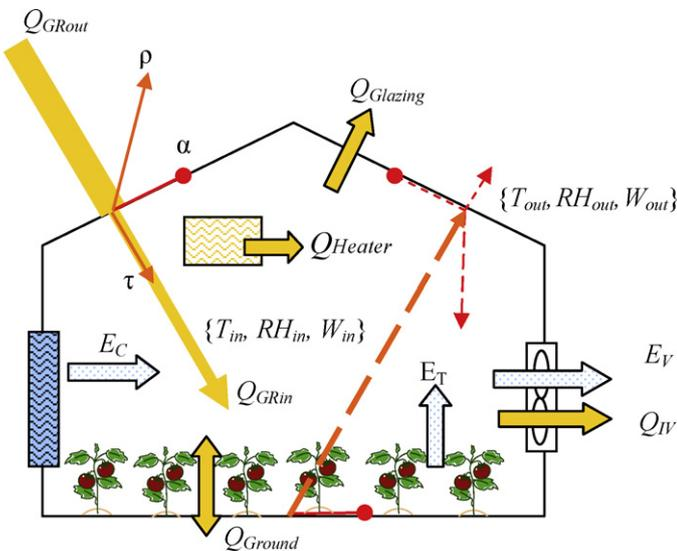
Fig. 3. Energy and water vapor fluxes within the greenhouse which define the energy and mass balance equations. See Table of Nomenclature for definitions of each parameter and variable.
