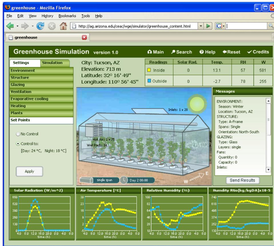
Fig. 4. Screen capture of the simulator after running a simulation of the greenhouse environment for winter conditions in Tucson, AZ.
